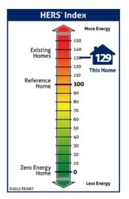
1 BR 1st Flr.- Unit 122 1 BR- prereno Community: N/A Conditioned Floor Area: 645 ft<sup>2</sup> Number of Bedrooms: Primary Heating System: Air Source Heat Pump • Electric • 7.7 HSPF Primary Cooling System: Air Source Heat Pump • Electric • 10 SEER Primary Water Heating: Residential Water Heater • Electric • 0.88 Energy Factor House Tightness: 2689 CFM50 (16.68 ACH50) Ventilation: None
