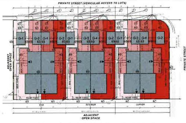
SPDX DETAIL: QUADRUPLEX TYPICAL LOT LAYOUT (ADJACENT OPEN SPACE AT REAR) SCALE 1" = 32'
