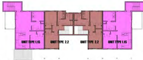
BUILDING TYPE F (2) TYPE 1.1 UNITS (2) TYPE 1.1S UNITS (2) TYPE 2.2 UNITS 3 2nd FLOOR - BLDG. F 10'-11"
