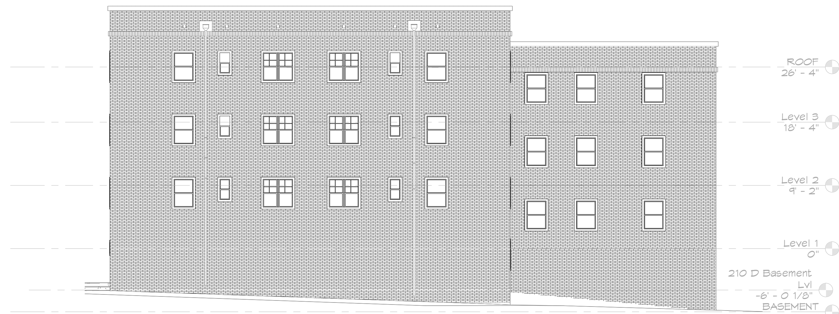
4 BUILDING 210 WEST ELEVATION (NEW WORK) A-304 SCALE: 1/8" = 1'-0"
